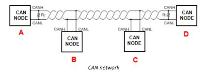
If the IOM6 CAN/LIN Accessory is connected at one of the ends of the network (node A or D in the diagram above) the 120 Ohm termination impedance can be enabled using the switch on the iSYSTEM connector accessories. If connected to the CAN bus at the position of nodes B and C, no termination is required.
