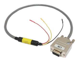
The IC57040-LIN-PIN cable is used to connect the IOM6-CAN/LIN to an existing LIN network to the pins typically found on a 2.54mm pitch header (0.63mm square pins). The cable length is 0.65m. The cable connects to the LIN1 or LIN2.
