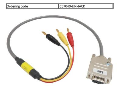
The IC57040-LIN-JACK cable is used to connect the IOM6 CAN/LIN Accessory to an existing LIN network via banana jack connectors. The cable length is 0.65m. The cable connects to the LIN1 or LIN2 connector.
