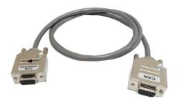
The IC57040-CAN-DB9 is used to connect the IOM6-CAN/LIN to an existing CAN network through the DB9 connector. 120 Ohm termination is selected with the switch located on one of the DB9 connectors. The cable length is 1m.
