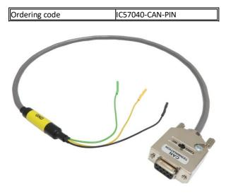
The IC57040-CAN-DB9 is used to connect the IOM6 CAN/LIN Accessory to an existing CAN network to the pins typically found on a 2.54mm pitch header (0.63mm square pins). The 120 Ohm termination impedance is selected using the switch located on the cable DB9 connector. Cable length is 0.65m.
