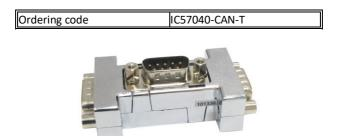
The IC57040-CAN-T is used to connect the IOM6 CAN/LIN Accessory to a CAN bus by splitting the existing bus connection – position F on the diagram below. The existing CAN bus connection is split using the IC57040-CAN-T allowing the IOM6 CAN/LIN Accessory to connect to it using an IC57040-CAN-DB9 cable (no termination required).
