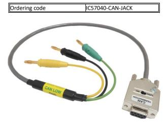
The IC57040-CAN-DB9 is used to connect the IOM6 CAN/LIN Accessory to an existing CAN network through the banana jacks. The 120 Ohm termination impedance is selected using the switch located on the cable DB9 connector. Cable length is 0.65m.
